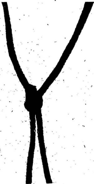
Figure 4-2: The projected area of a knot made from 3 mm polyethylene twine. Scale, twice actual size.
