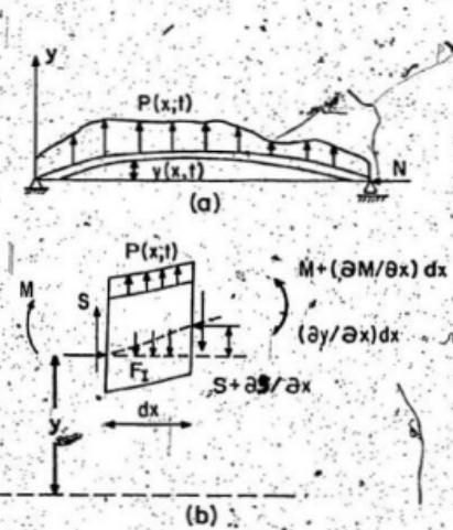
Fig. 5.1 Beam with Static Axial Force and Dynamic Lateral Load a) Beam Deflection Profile b) Forces on Differential Element
