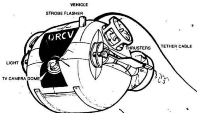
Figure 4.2: HydroProducts RCV-225
