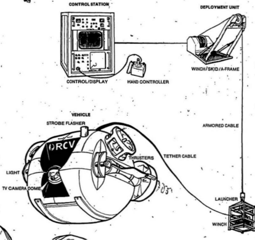
Figure A.1 : Hydro Products RCV-225
