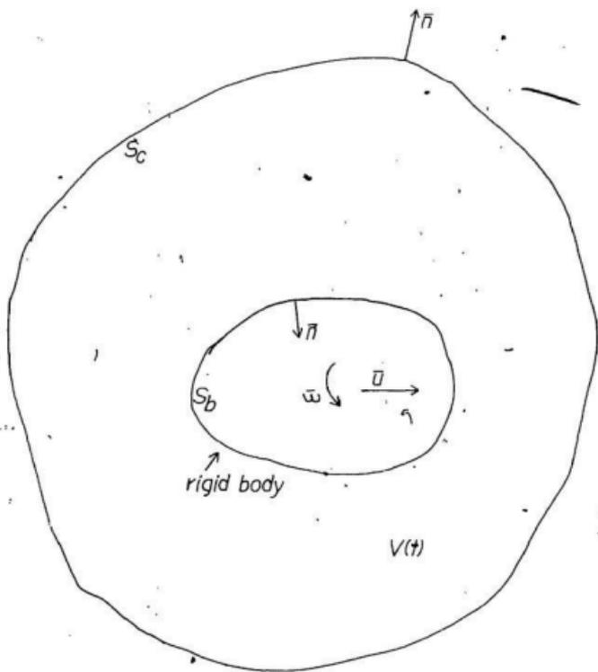
Figure 3.1: Rigid Body and Control Surfaces
