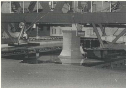
Figure 3.1 Experimental set-up showing a 1:25 scale large neck model mounted under the main carriage
