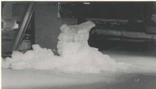
Figure 4.2 Photo from IMD's series showing the ride-up of ice and the rubble pile (Test MUNCONE6_003)
