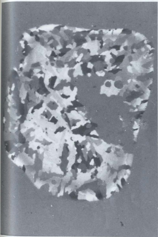
FIGURE 16 - Thin Section From Middle Depth of an Ice Block.
