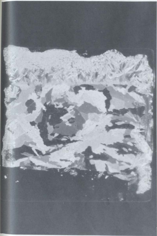
FIGURE 17 - Thin Section from Bottom of an Ice Block.
