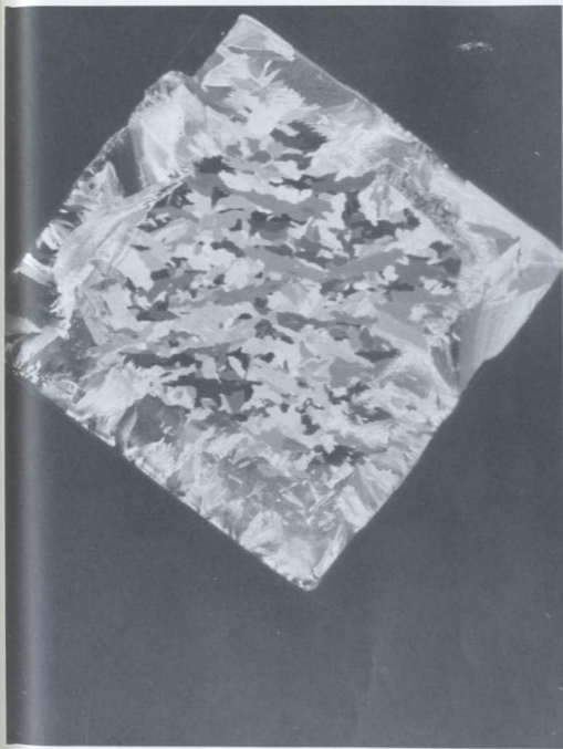
FIGURE 15 - Thin Section From Top of an Ice Block.
