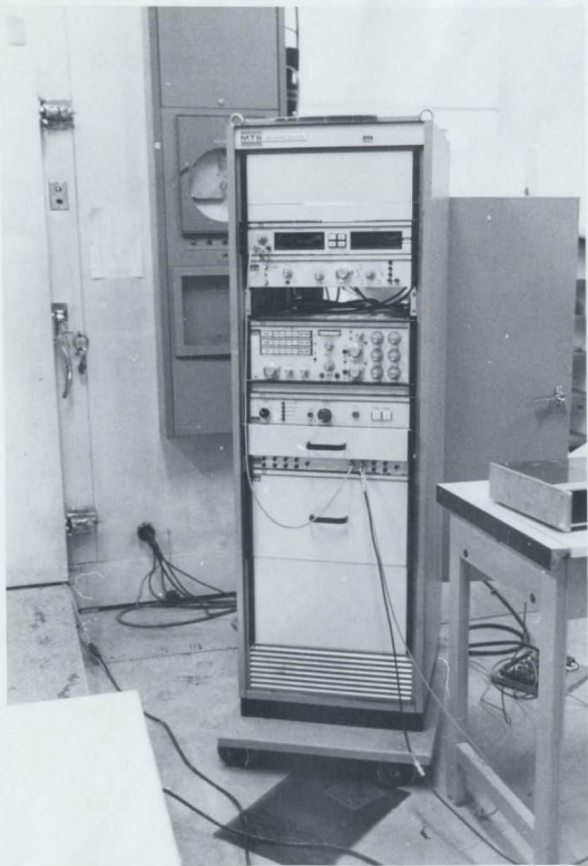
FIGURE 4(b) The Control Console of N.T.S. Machine Outside The Coldroom.
