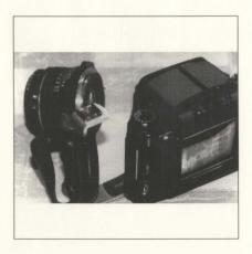
Light shines on a subject, reflects toward the camera, and enters the lens. The lens then focuses this light onto the film forming an image.
