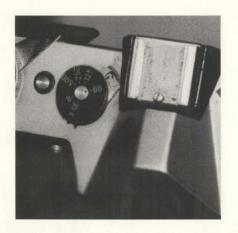
Shutter speeds range from around 1s to 1/2000s on modern 35mm cameras and like f-stops, each successive increment is 1/2 of the previous value, approximately. Common shutter speeds given in fractions of a second are: 1/2, 1/4, 1/8, 1/15, 1/30, 1/60, 1/125, 1/250, 1,500, and 1/1000.
