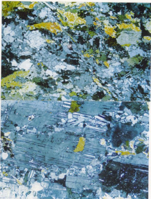
Fig. 3.25.- Microtexture of the 557 Ma Sandbank Point metagabbro/diorite. Top: D2 greenschist overprint of the earlier metamorphic fabric. Note: grain reduction, growth of chlorite and brittle offset of amphibole along a discrete shear band (Arrow). Other deformational features are discussed in the text. Field of view is 5.21 mm wide. Bottom: mantle-core structure in plagioclase with subgrain rotation recrystallization. Field of view is 1.32 mm.
