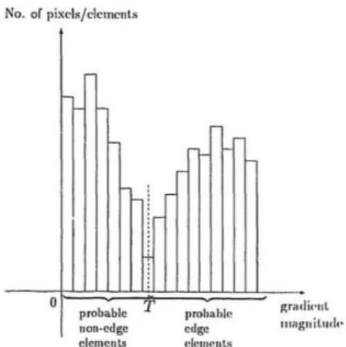
Figure 3.4 Threshold determination from gradient magnitude histogram
