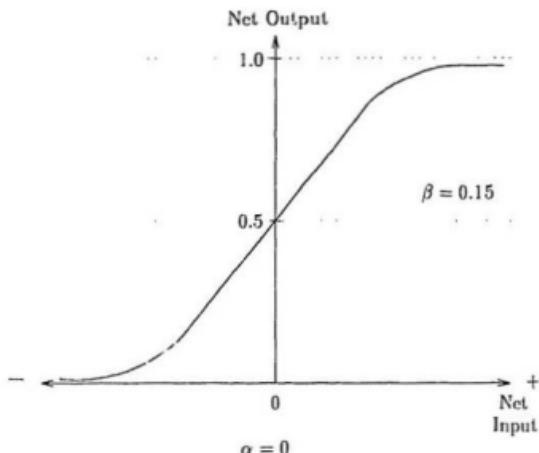
Figure 4.11 Characteristics of sigmoidal activation function
