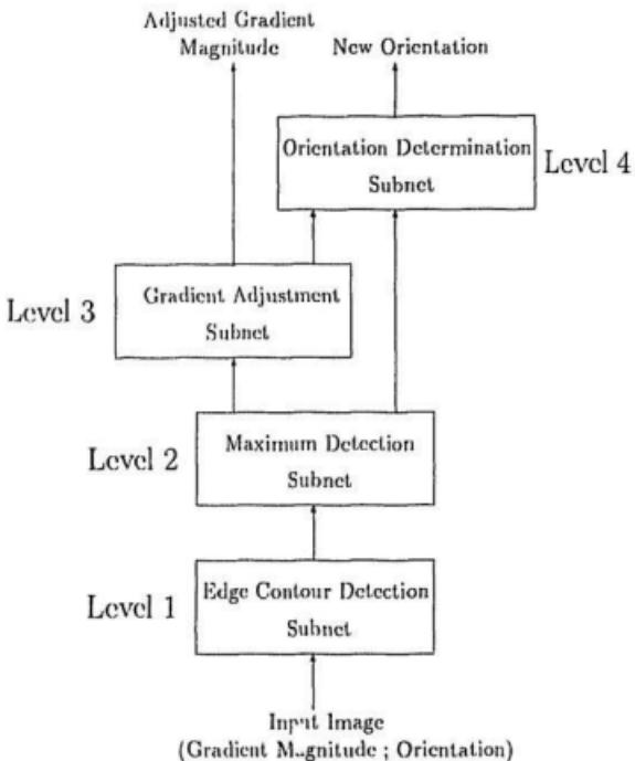
Figure 1.2 Hierarchical structure of neural network system
