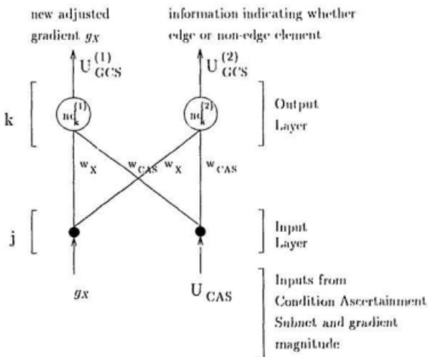
Figure 6.4 Architecture of Gradient Computation Subnet
