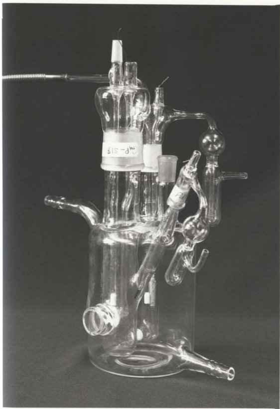
Figure 6b. The jacketed photoelectrochemical cell equipped with, front, a semiconductor electrode, to its right, a palladium reference electrode, and behind, a platinum counter electrode.
