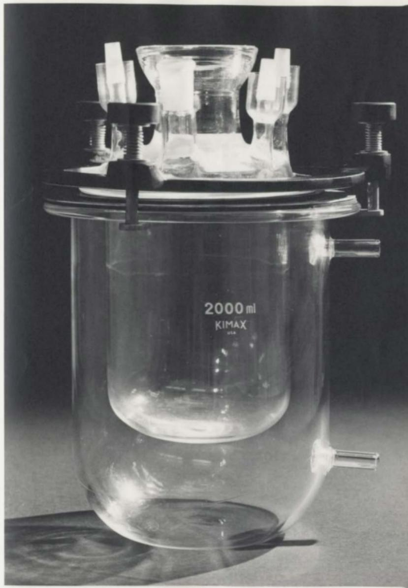
Fig. 6 The cell, mounted in its thermostating jacket.
