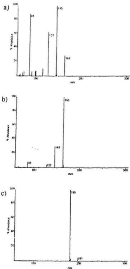
**Figure 4.12:** Chemical Ionization (CI) Mass Spectra of Levoglucosan using different reagent gases. (a) Methane, (b) n-Isobutane and (c) Ammonia.
