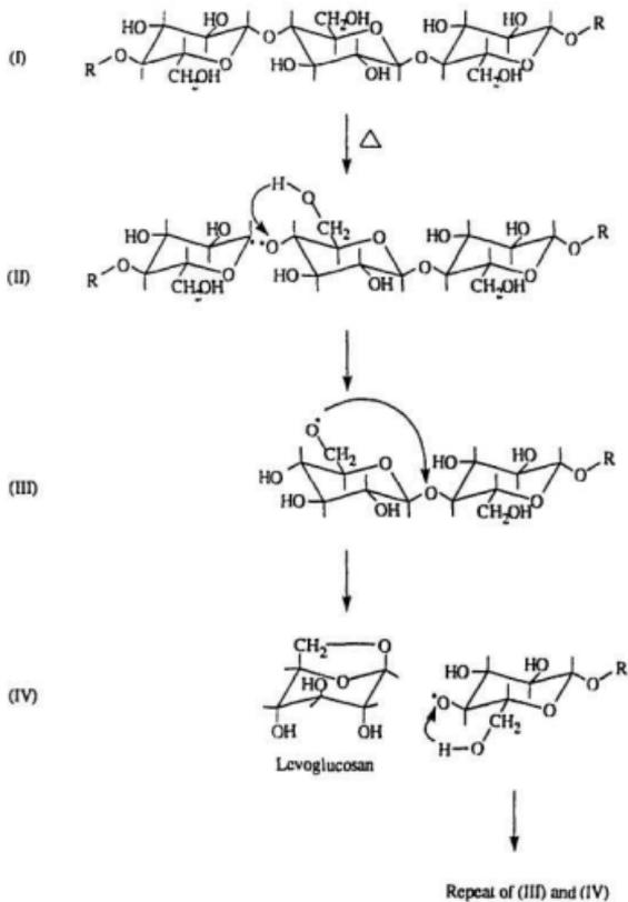
Figure 1.7: Homolytic Fission of Cellulose (72).
