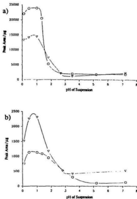
Figure 4.6: The Influence of Suspension pH on the Anhydrosugar Yields for Black Spruce Mechanical (v) and Kraft (o) Pulps, (a) Anhydroglucoses ar:<sup>1</sup> (b) 1,4-Anhydroxylopyranose.
