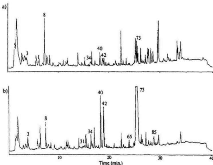
Figure 4.2: Pyrograms of Birch Mechanical Pulp (a) Untreated and (b) Acid-Washed.
