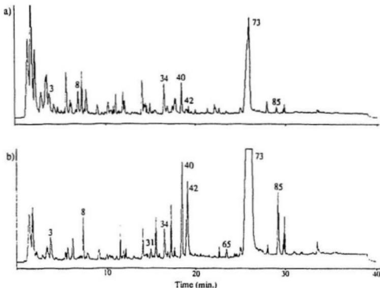
Figure 4.4: Pyrograms of Birch Alcell® Pulp (a) Untreated and (b) Acid-Washed.
