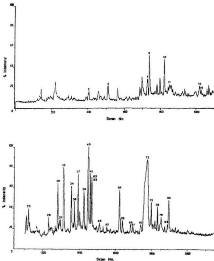
Figure 4.14: Total Ion Chromatogram (TIC) for Acid-Washed Birch Mechanical Pulp obtained by Py-GC-MS(NH<sub>3</sub>-Cl).
