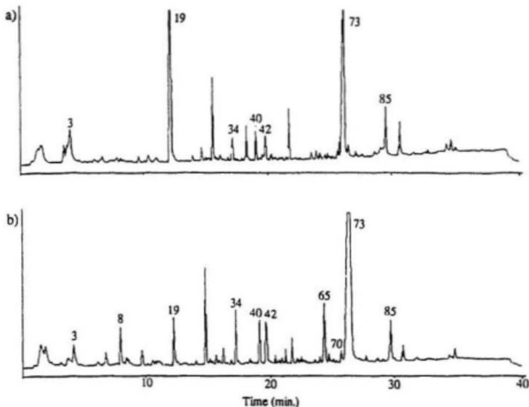
**Figure 5.3:** Pyrograms of Noranda Sulfite Pulp (N.S.P. #231090) (a) Acid-Washed and (b) Fe<sup>2+</sup>-Exchanged.
