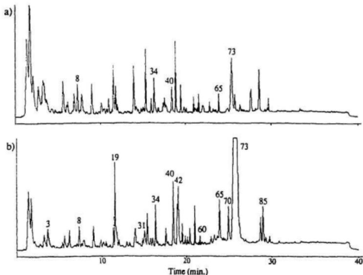
**Figure 4.1:** Pyrograms of Black Spruce Mechanical Pulp (a) Untreated and (b) Acid-Washed.
