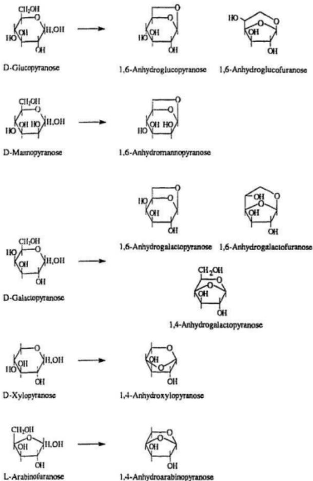
Figure 1.11: The Saccharides Found in Wood and The Anhydrosugars They Form Upon Pyrolysis.
