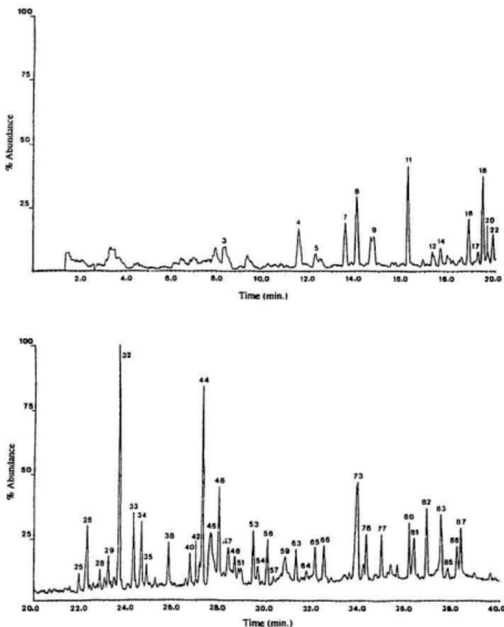
**Figure 5.4:** Total Ion Chromatogram (TIC) of Untreated Noranda Spruce Sulfite Pulp
