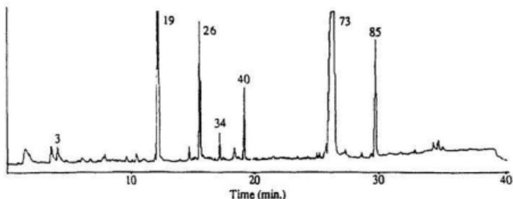
Figure 5.2: Pyrogram of Avicel Microcrystalline Cellulose sorbed with dilute  $H_2SO_4$ .
