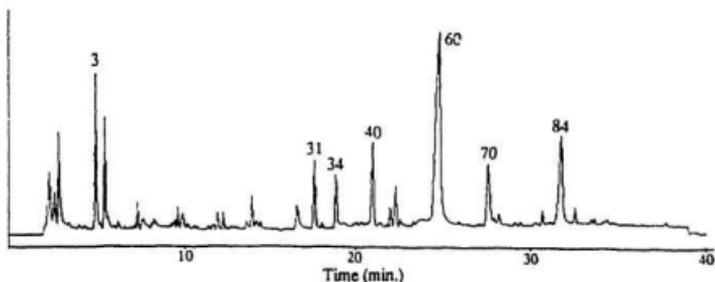
Figure 3.4: Pyrogram of Proton-Exchanged Arabinogalactan.
