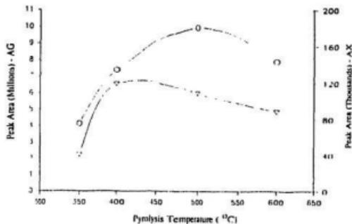
**Figure 6.1:** The Effect of Pyrolysis Temperature on the Anhydrosugar Yields for Glucose (○) and Xylose (▼) from Acid-Washed Black Spruce Mechanical Pulp.
