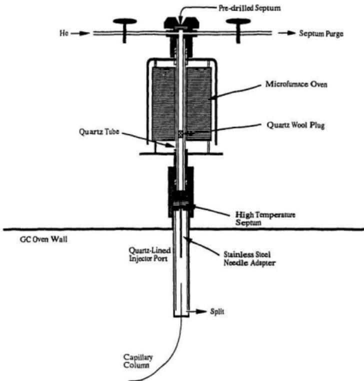
Figure 2.2: SGE Pyrojector<sup>®</sup>
