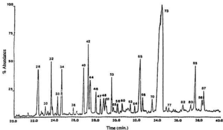
Figure 5.7: Total Ion Chromatogram (TIC) for Fe<sup>2+</sup>-Exchanged, Noranda Spruce Sulfite Pulp
