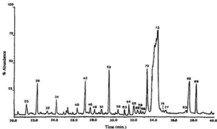
Figure 5.5: Total Ion Chromatogram (TIC) of Acid-Washed Noranda Spruce Sulfite Pulp
