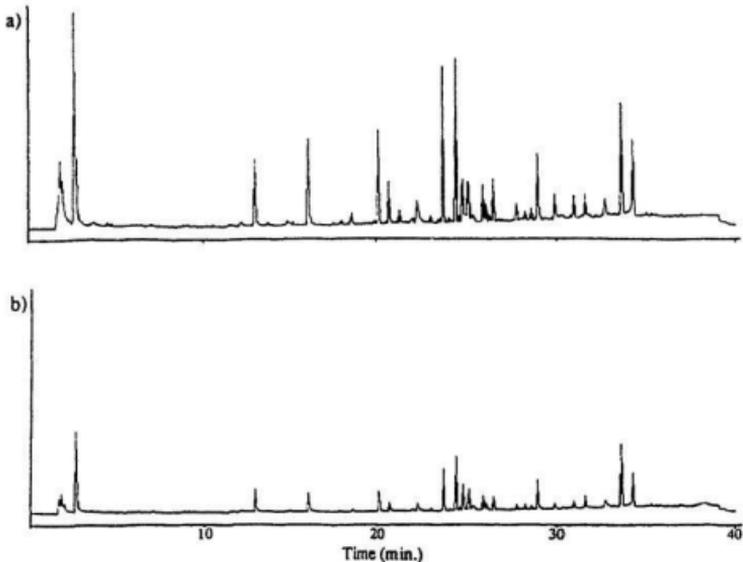
**Figure 4.8:** Pyrograms of Spruce Milled Wood Lignin (a) Untreated and (b) Acid-Washed.
