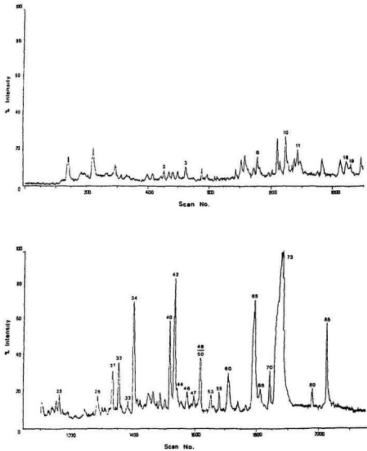
Figure 4.13: Total Ion Chromatogram (TIC) for Acid-Washed Black Spruce Mechanical Pulp obtained by Py-GC-MS(NH<sub>3</sub>-Cl).
