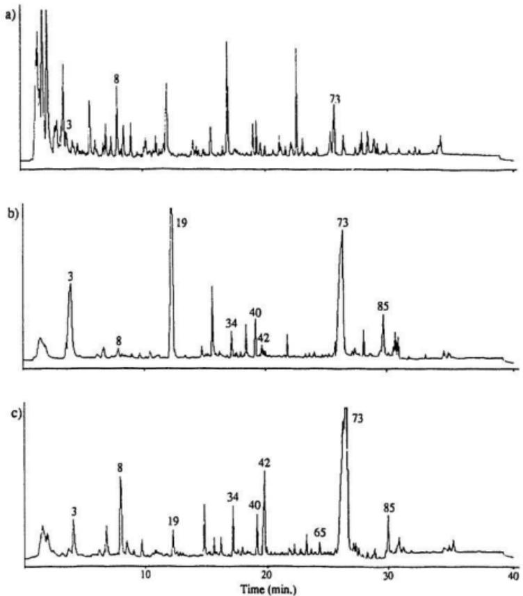
**Figure 5.1:** Pyrograms of Aspen Steam Explosion Pulp (a) Untreated, (b) Acid-Washed and (c)  $\text{Fe}^{2+}$ -Exchanged.
