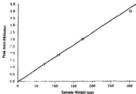
**Figure 6.4:** Sample Weight versus Anhydroglucose Peak Area (73 + 85) for Avicel Microcrystalline Cellulose using the Pyrojector®.
