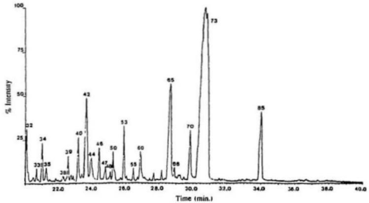
Figure 4.11: Total Ion Chromatogram (TIC) for Acid-Washed Birch Mechanical Pulp Obtained by Py-GC-MS(EI).
