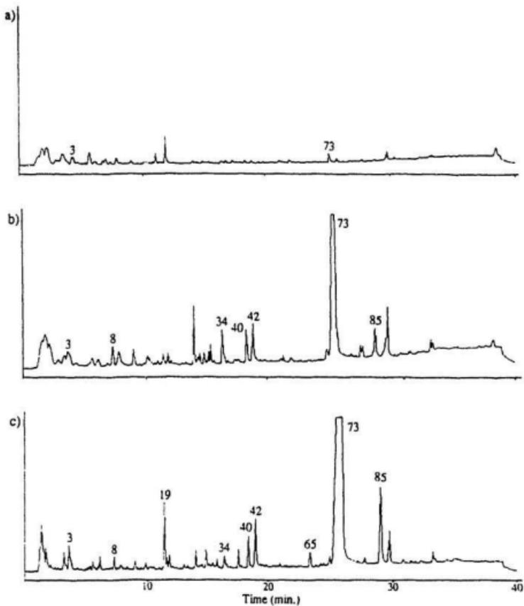
**Figure 4.5:** Pyrograms of Acid-Washed Black Spruce Kraft Pulp Treated with (a) 0.1 N KCl, (b) 0.1 N  $\text{CaCl}_2$  and (c) 0.1 N  $\text{FeCl}_2$ .
