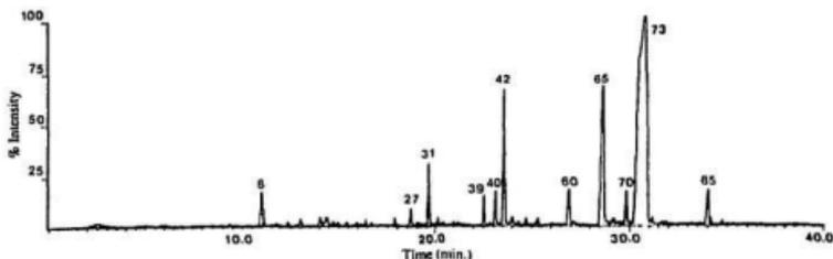
Figure 7.1: Extracted Ion Chromatogram ( $m/z$  57) for Acid-Washed Black Spruce Mechanical Pulp.
