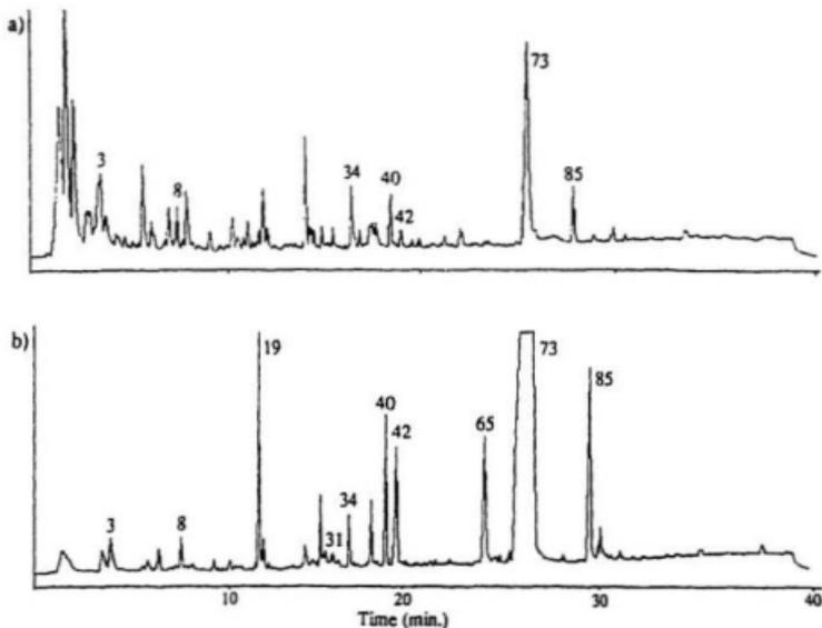
Figure 4.3: Pyrograms of Black Spruce Kraft Pulp (a) Untreated and (b) Acid-Washed.
