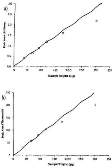
**Figure 6.2:** Linear Dynamic Range Curves for Anhydrosugar Production for Acid-Washed Black Spruce Mechanical Pulp, (a) Anhydroglucoses and (b) 1,4-Anhydroxylopyranose.
