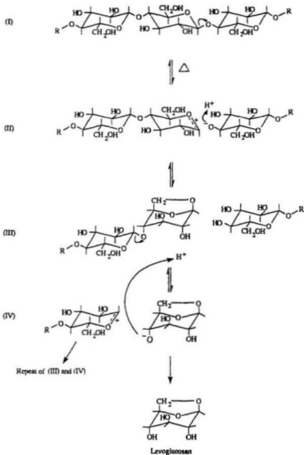
Figure 1.8: Heterolytic Fission of Cellulose (73).
