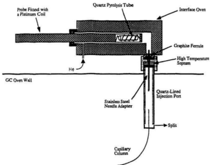
Figure 2.1: CDS Pyroprobe 120<sup>®</sup>.
