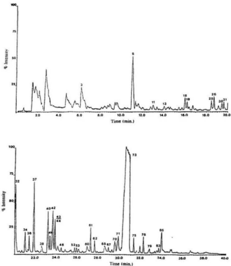
Figure 4.10: Total Ion Chromatogram (TIC) for Acid-Washed Black Spruce Mechanical Pulp
