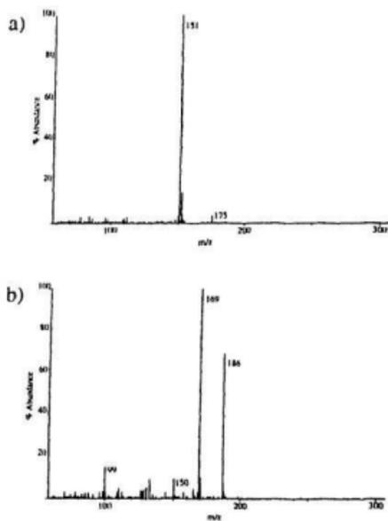
Figure 4.15: Ammonia Chemical Ionization Mass Spectra of (a) 4-Vinyl Guaiacol, 32, and (b) 4-Methyl Syringol, 43.
