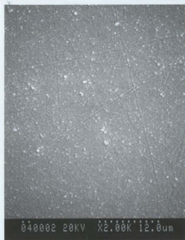
Figure 3.16 Scanning electron micrographs for the polymer film prepared on a rotating electrode at 1600 rpm as shown in Figure 3.7d. Polymerization time: 3 min.
