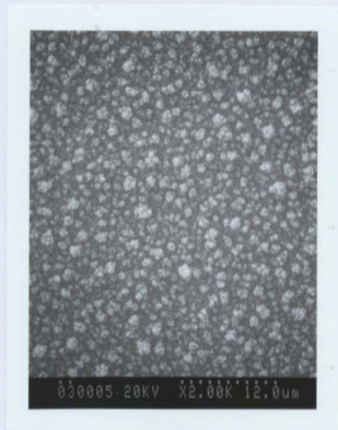
Figure 3.15 Scanning electron micrographs for the polymer film prepared on a rotating electrode at 900 rpm as shown in Figure 3.7c. Polymerization time: 3 min.
