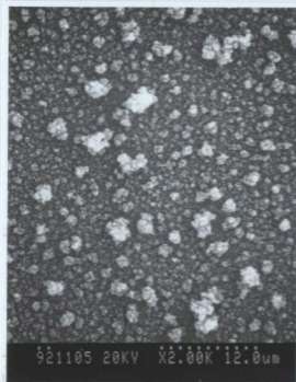
Figure 3.17 Scanning electron micrographs for the polymer film prepared on a stationary electrode under the experimental conditions as shown in Figure 3.7, but the polymerization time was 1.5 min.
