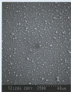
Figure 3.18 Scanning electron micrographs for the polymer film prepared on a rotating electrode at 400 rpm under the experimental conditions as shown in Figure 3.7, but the polymerization time was 1.5 min.
