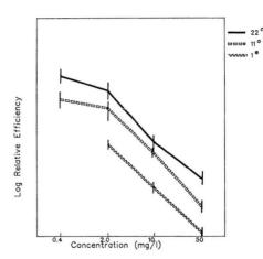
Fig. 27. Relationship of relative feeding efficiency and PM concentration at two temperatures, for <u>P. mixtum</u> larvae (mean ± 1 s.e.), at 9 cm/s current velocity.
