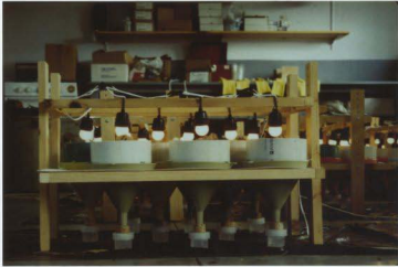
Figure 7: Modified Berlese funnel apparatus used for extracting soil samples from fir ( Abies balsamea ) - fern ( Dryopteris ) and fir - horsetail ( Equisetum ) forest sites.
