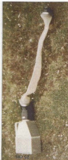
Figure 4.1: Dredge sampler used in quantitative sampling regime. The opening at the left is 25 cm.
