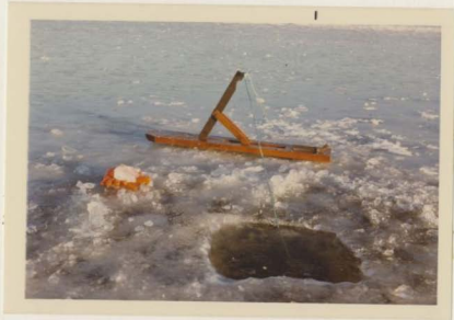
Fig. 7. Prairie-ice jigger used to set gill nets beneath the ice.
