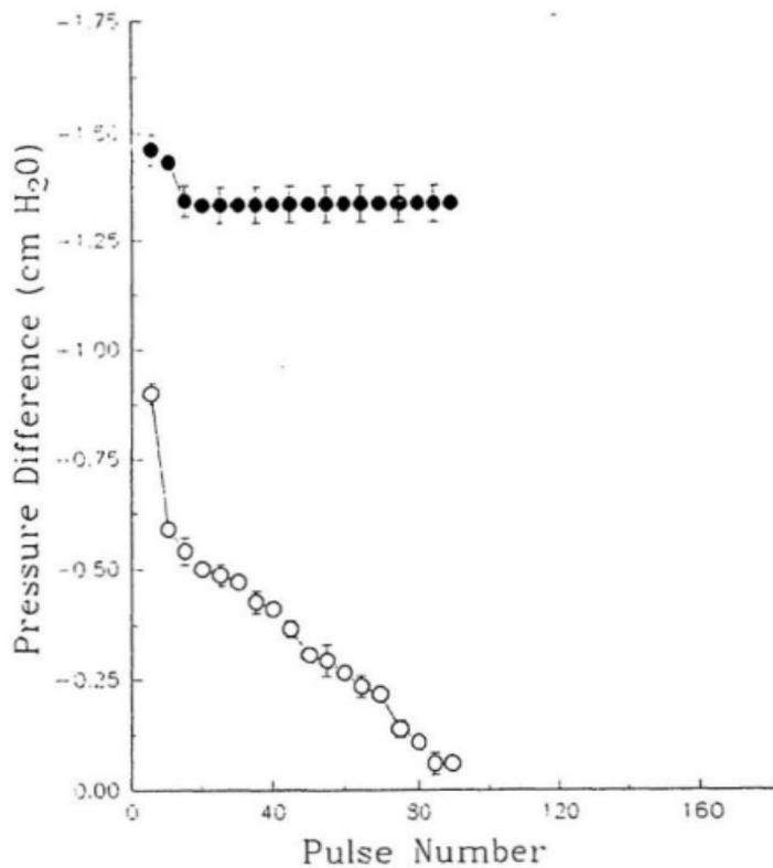
Figure 22. Reductions of bubble surfactometer tracings for a suspension of albumin ( $0.10 \text{ mg} \cdot \text{ml}^{-1}$ ) + porcine lipid extract surfactant ( $1.0 \text{ mg} \cdot \text{ml}^{-1}$ ) which was suspended in water which contained  $0.15 \text{ M NaCl}$  and  $0.005 \text{ M CaCl}_2$ ,  $n=5$ .
