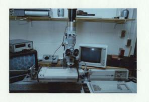
Images could be either captured directly from the camera through the TARGA board and stored through a specially written macro programme, or recorded with the VCR and digitized from the tape. Initial size calibration was done using a micrometer scale giving 0.2 \( \mu\)pixel of spatial resolution.
