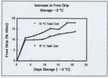
Figure 3-13: Influence of storage of cod muscle at  $0^{\circ}\mathrm{C}$  or  $10^{\circ}\mathrm{C}$  on free drip
