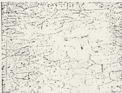
Fig. 19. 4% Nital x 300 Structure of cold worked wrought iron: lightly elongated ferrite grains.
