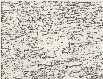
Fig. 22. 4% Nital x 300 Structure of cold worked medium carbon steel (0.3%C): elongated grains of ferrite (light) and pearlite (dark) in object 1-1.
