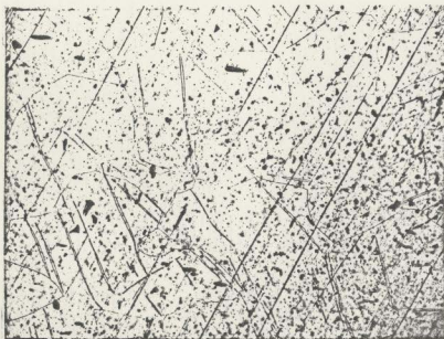
Fig. 21. 4% Nital x 160 Structure of wrought iron nail head resulting from a hammer blow: equiaxed ferrite grains crossed with Neumann bands.
