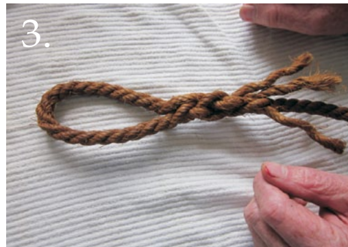
Guy Bussey in St. Lunaire-Griquet splicing three-strand rope.
