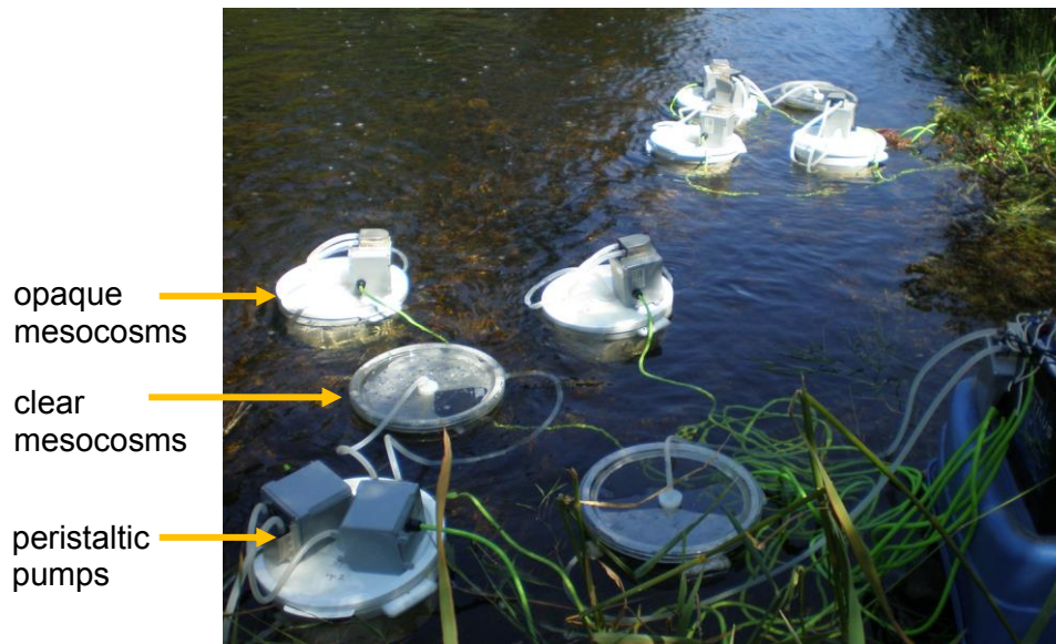
Figure A4.1: Experimental set-up of the mesocosm experiments described in detail in the method section in chapter 4. Clear (light) and opaque (dark) 12 L polycarbonate enclosures, equipped with peristaltic pumps to maintain stream water circulation, were filled with stream water substrate (6 – 7 rocks each) randomly collected from the stream at each study site. Eight liters of unfiltered stream water, initially spiked with ^{13}\text{C} -labeled bicarbonate as a tracer for autochthonous carbon generated during the experiments, were added to the mesocosms.
