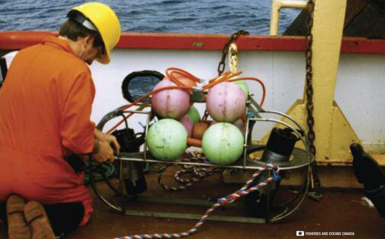
Figure 2: Gear technologist preparing a camera system for deployment.
