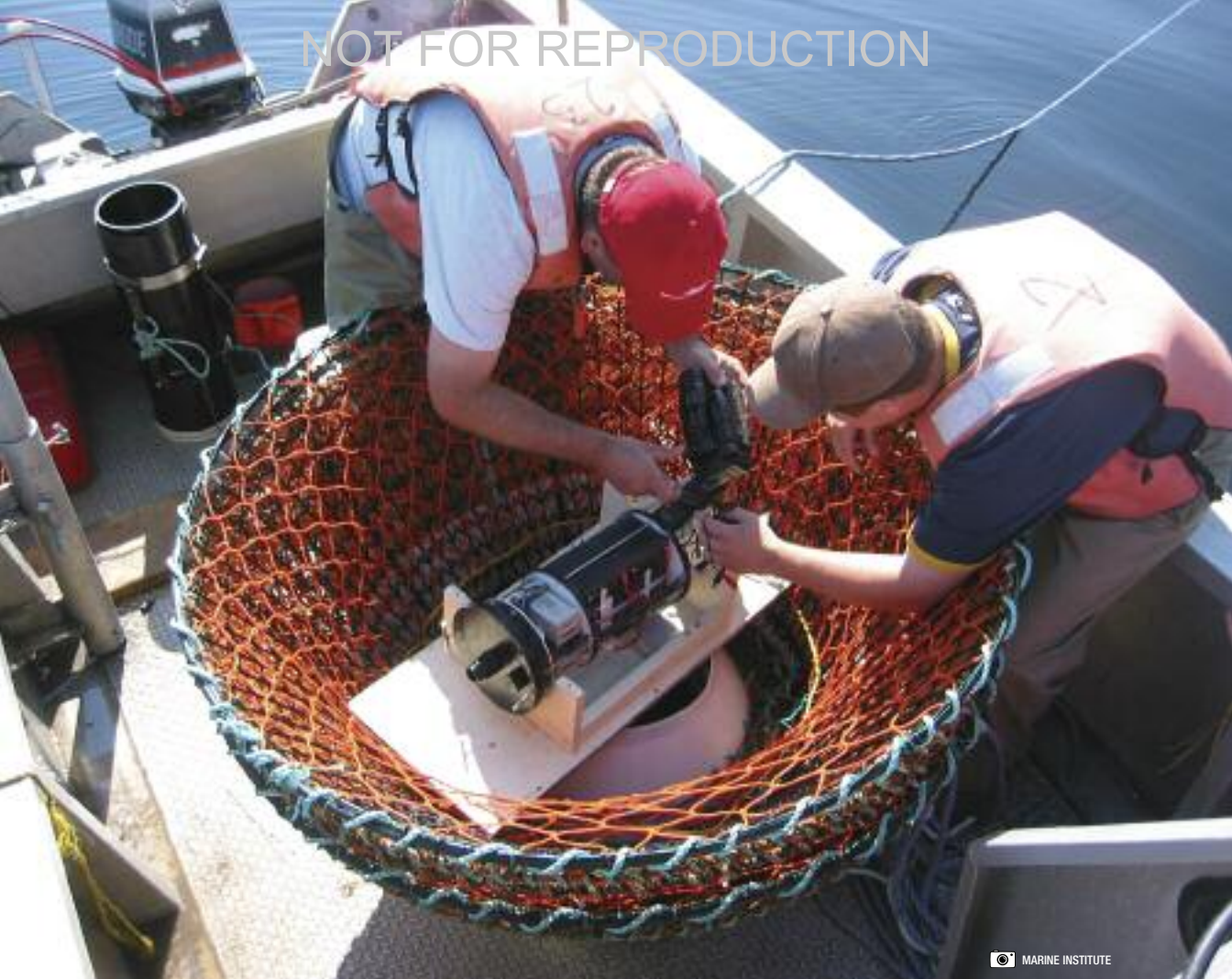
Figure 4: Preparing a self-contained underwater recording bottle.
