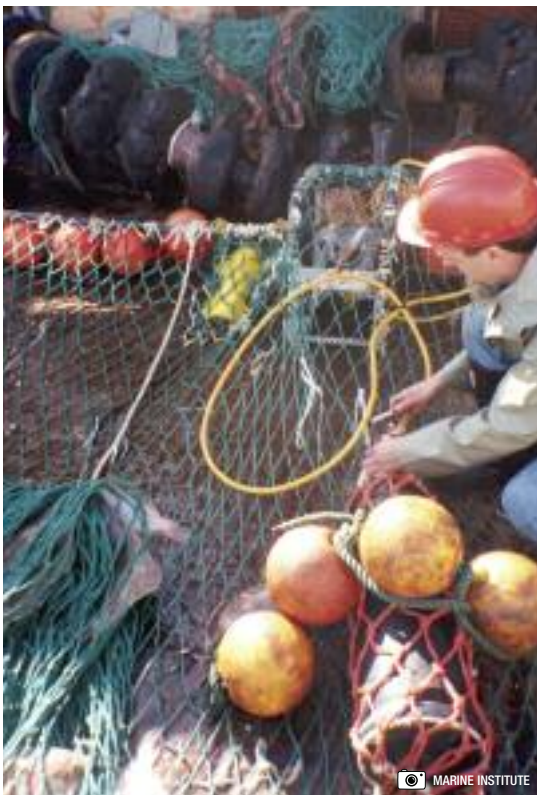
Figure 5: Attaching a camera and recording bottle to the headline of a bottom trawl.
