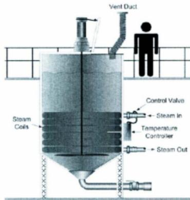
Figure 6.6. Mixing tank and safety measures (CSB, 2007).
