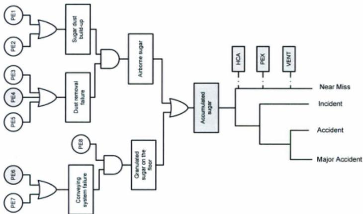
Figure 5.3. Bow-tie modeling of sugar dust explosion at Imperial Sugar manufacturing facility
