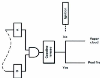
Figure 6.2. Bow-tie model for gasoline release accident scenario. For the sake of brevity, the fault tree part is not completely illustrated
