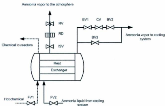
Figure 7.12. Schematic of the heat exchanger in the Goodyear accident (CSB, 2011).
