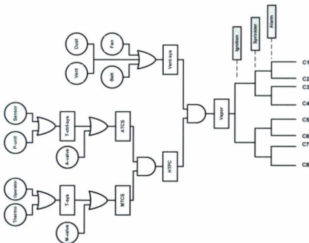
Figure 6.7. BT model for the heat exchanger accident scenario (CSB, 2007).
