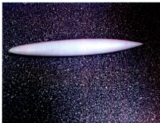
Figure A.1: 3D Printed NACA Airfoil: Printed using a rapid prototype machine, sprayed with a filler and sanded.
