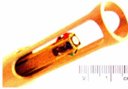
Figure 2-4: Acoustic Velocity Sensor [16]
