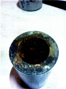
Figure 6.19 – Rust observation on the prototype surfaces: (a) orifice, (b) exterior, (c) inlet
