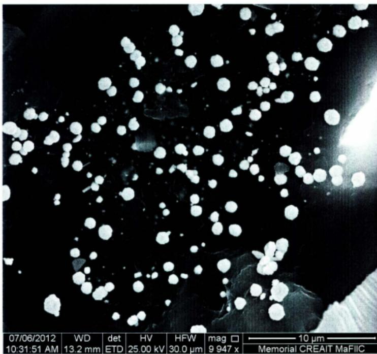
Figure 9.20:SEM photograph of cloth adsorbent gel after gold adsorption. Magnification:10000X
