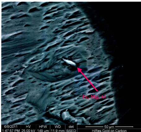
Plate 5: High magnification backscatter electron image of an inclusion containing iron (Fe), magnesium (Mg) and aluminium (Al) in a gypsum crystal.
