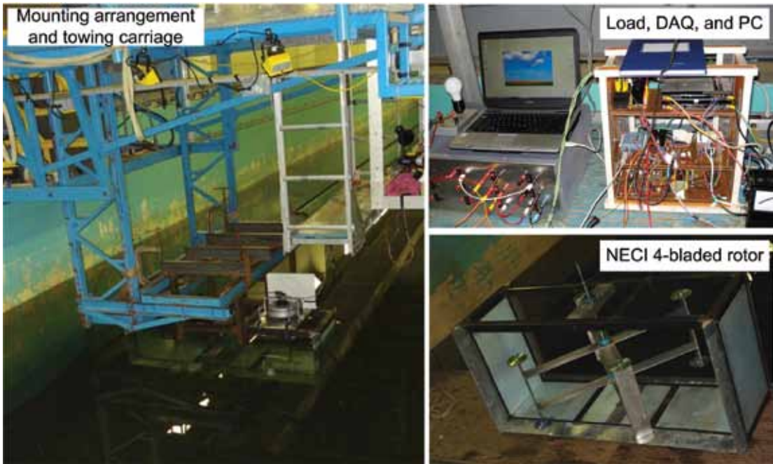
Figure 5: Rotor mounting and test arrangement.
