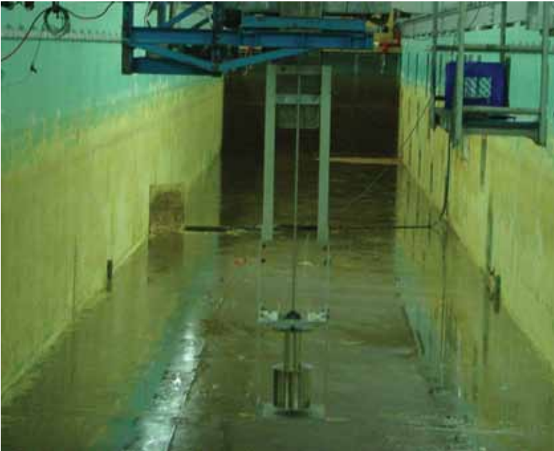
8b: Set up of the frame and rotor in the wave tank.
