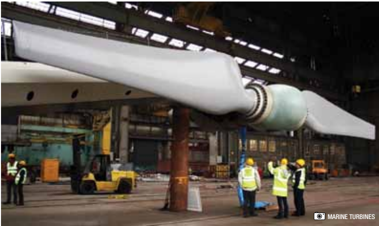
Figure 1: A 600 kW marine current generator.
