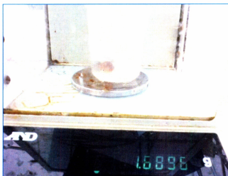
Figure 6. Weight measurement on a plate with a four d.p. electronic balance.
