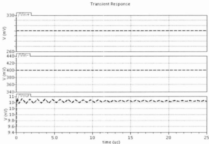
Figure 42: Transient Simulation Result for two stage open loop comparator with  $V_{in}^+ = 0.3V$  and  $V_{in}^- = 0.4V$  in TSMC 0.18 $\mu m$  technology
