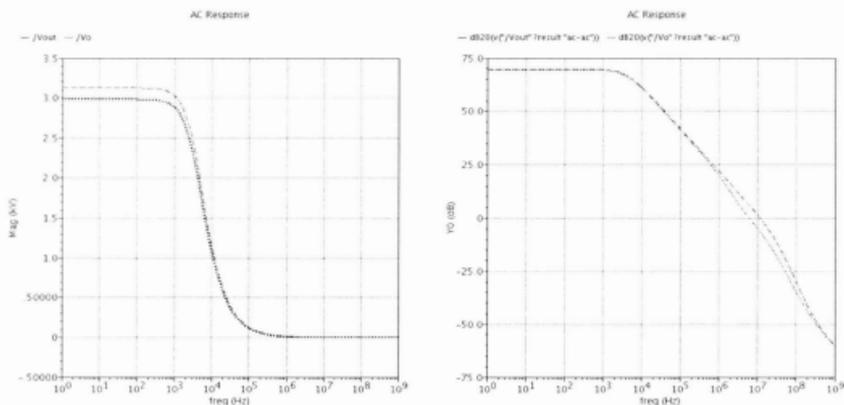
**Figure 28: Pre-layout in Cadence for Two Stage PMOS Op Amp in TSMC 90nm technology. (Red-dashed: Design with interconnect parasitics in consideration, blue-dotted-without consideration)**
