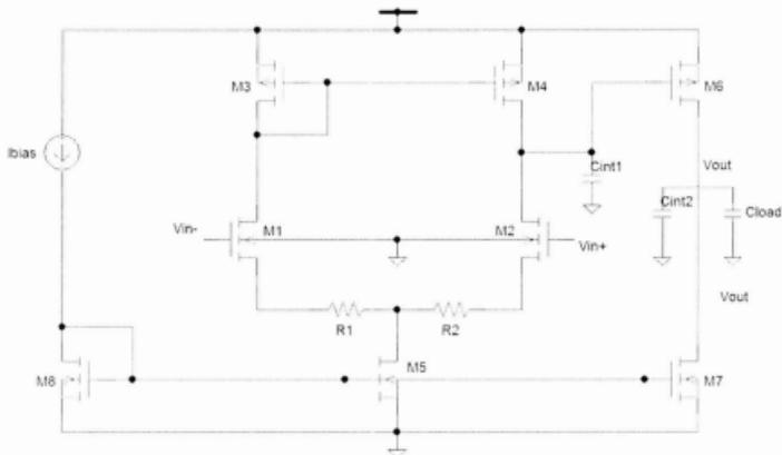
Figure 40: Two Stage Open Loop Comparator [27].
