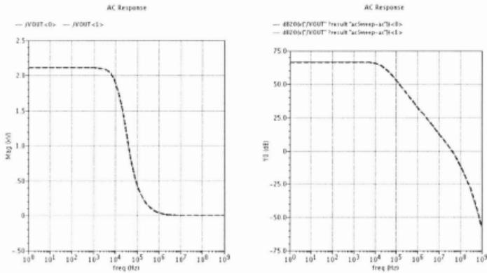
**Figure 39:** Post layout simulation result for Cascode Two Stage Amplifier in Cadence TSMC 0.18 $\mu$ m technology. (Magenta-Solid: Post Layout Simulation, Red-Dashed-Prelayout Simulation)
