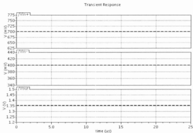
Figure 41: Transient Simulation Result for two stage open loop comparator with  $V_{in+} = 0.7V$  and  $V_{in-} = 0.4V$  in TSMC 0.18um technology
