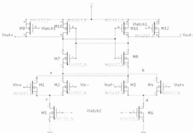
Figure 48: Differential Pair Comparator [10].
