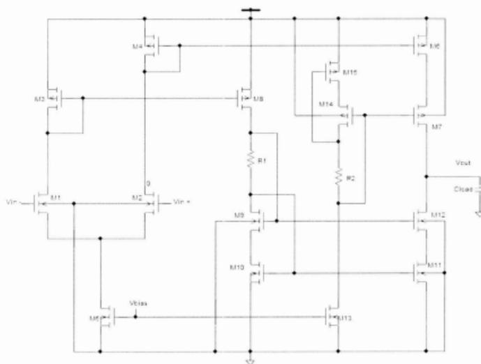
Figure 33: Cascode Two Stage Amplifier [27].
