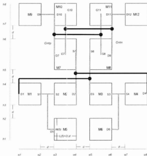
Figure 49: Differential Pair Comparator floorplan used to model interconnect parasitics
