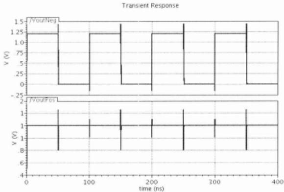
**Figure 4: The symmetric Differential Pair Post-layout simulation in TSMC 90nm for  $V_{in}^+ = 0.8V$  and  $V_{in}^- = 0.4V$**
