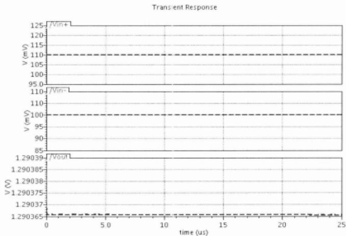
**Figure 43: Transient Simulation Result for two stage open loop comparator with  $V_{in+} = 110$  mV and  $V_{in-} = 100$  mV in TSMC 0.18um technology**
