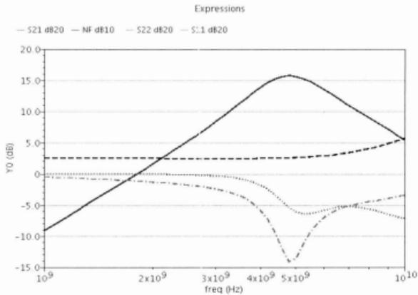
**Figure 58: Simulation result of CS inductively degenerate LNA design without considering parasitics. (Red-solid: S21 (gain), Blue-dashed: NF, Green-dot dash: S11, Pink-dotted: S22)**
