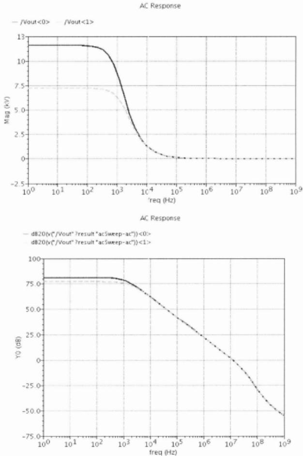
**Figure 21: Pre-layout in Cadence for Two Stage NMOS Op Amp in CMOS 0.18um Technology. (Magenta-Solid: Design with interconnect parasitics, Red-Dashed: Design without interconnect parasitics)**
