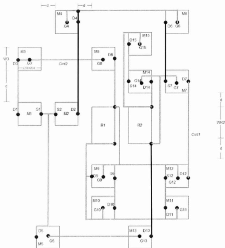
Figure 34: Floorplan for the Cascode Two Stage Amplifier.
