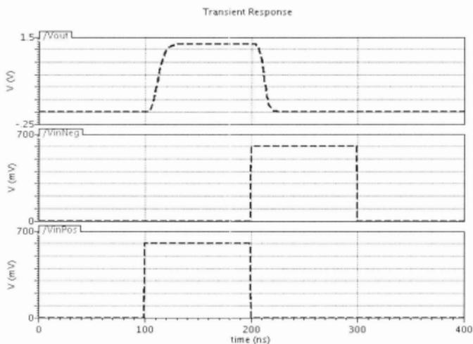
**Figure 44: Transient Simulation Result for two stage open loop comparator with PWL sources**
