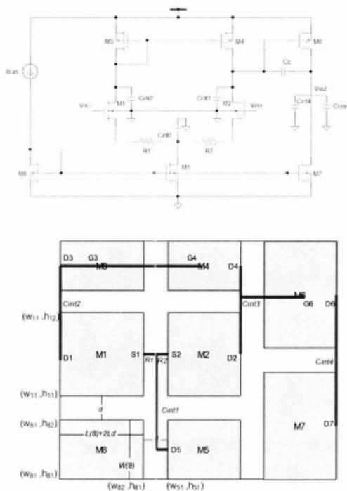
Figure 20: Schematic and Floorplan of Two Stage N-input Op Amp.
