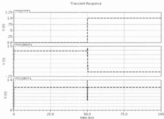
Figure 50: Differential Pair Pre-layout simulation in TSMC 90nm for  $V_{in}^+ = 0.8V$  and  $V_{in}^- = 0.4V$
