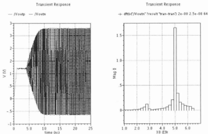
**Figure 62: Simulation Result for approximated total capacitance of  $251.29fF$  for LC oscillator in TSMC 90nm.**
