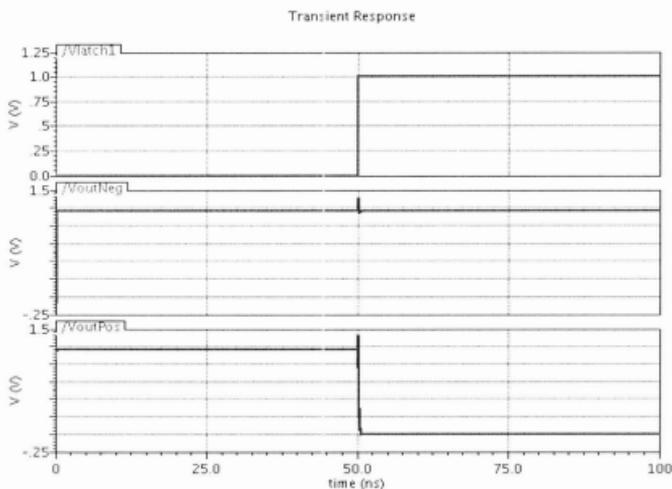
**Figure 55: Differential Pair Post-layout simulation in TSMC 90nm for  $V_{in}^+ = 0.3V$  and  $V_{in}^- = 0.4V$**
