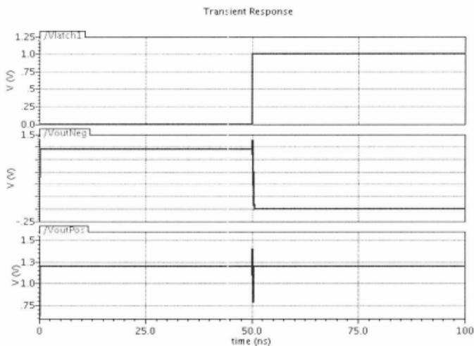
Figure 54: Differential Pair Post-layout simulation in TSMC 90nm for  $V_{in}^+ = 0.8V$  and  $V_{in}^- = 0.4V$
