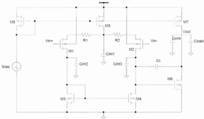
Figure 26: Two Stage P-input Amplifier [23].
