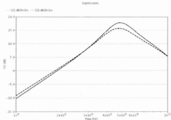
Figure 60: Gain Comparison of Source Degenerated LNA design with and without considering parasitics. (Solid-Red: With parasitics, Dashed-Blue: Without parasitics)
