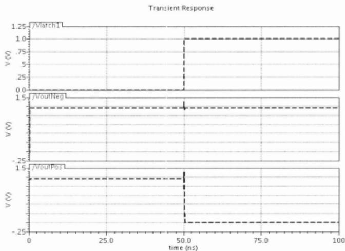
Figure 51: Differential Pair Pre-layout simulation in TSMC 90nm for  $V_{in}^+=0.3V$  and  $V_{in}^-=0.4V$
