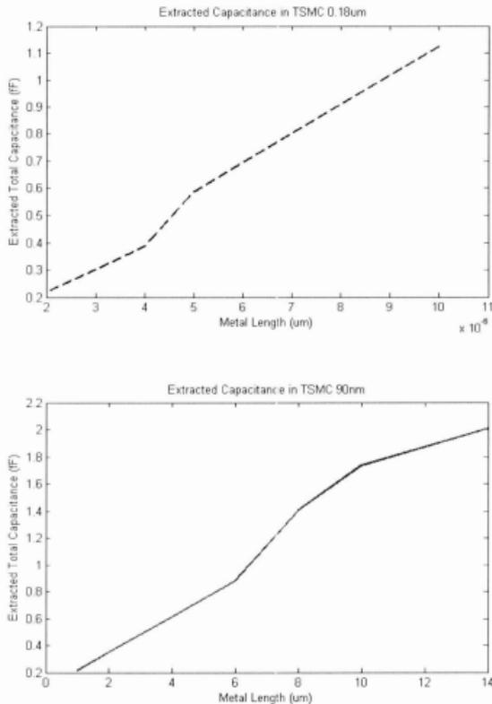
**Figure 15: Extracted Total Capacitance plotted in terms of Metal length.**
