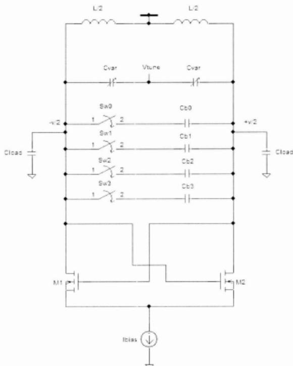
Figure 61: Cross Coupled LC Oscillator [36].
