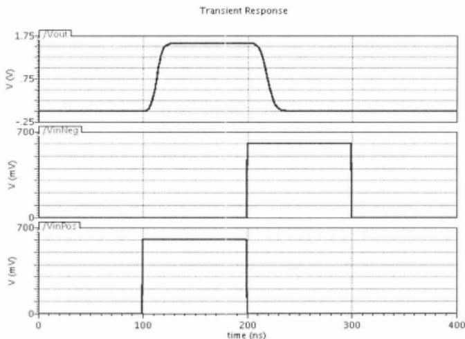
**Figure 47: Post layout transient simulation result for Open Loop Comparator**
