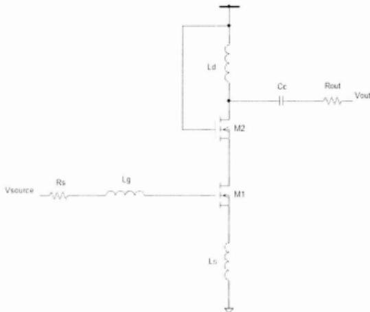
Figure 56: Cascode Common Source LNA with inductive degeneration [30].
