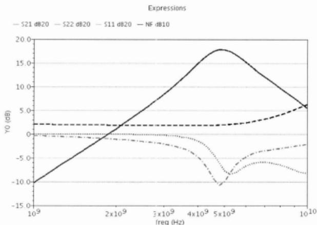
**Figure 59: Simulation result of CS inductively degenerate LNA design with considering parasitics. (Red-solid: S21 (gain), Blue-dashed: NF, Green-dot dash: S11, Pink-dotted: S22)**
