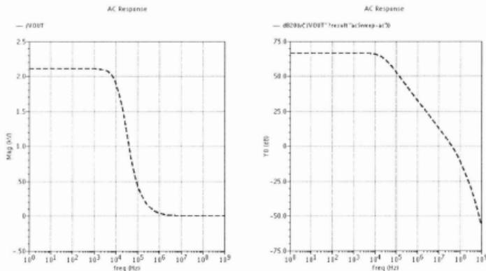
Figure 35: Simulation Result of Cascode Two Stage Amplifier in *TSMC 0.18um* technology
