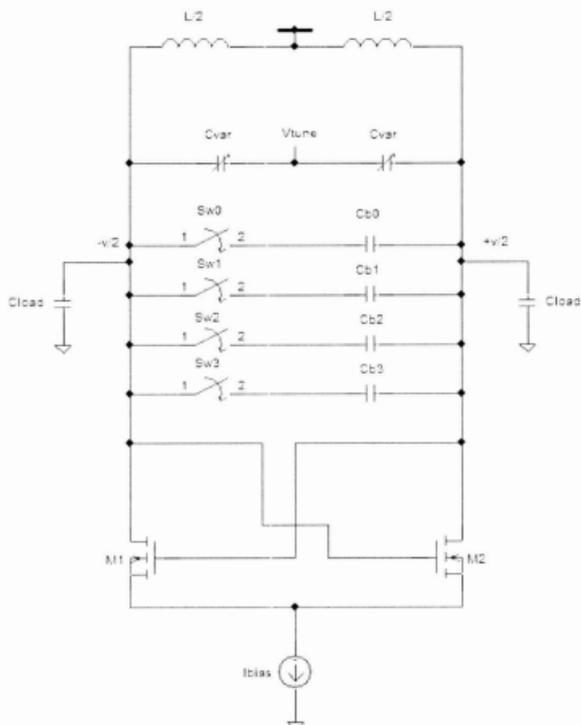
Figure 61: Cross Coupled LC Oscillator [36].
