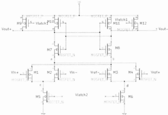
**Figure 2: Dynamic Comparator (Differential Pair Structure) [10].**
