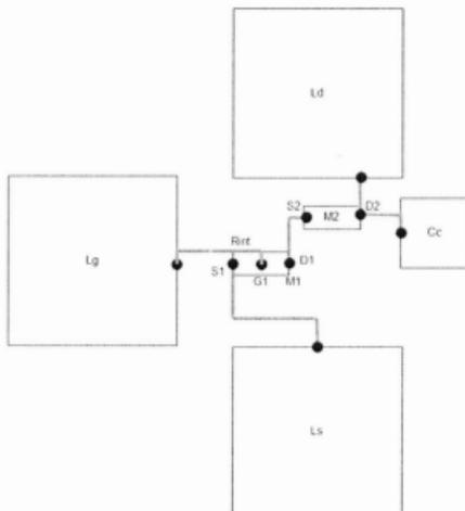
Figure 57: Floorplan for LNA to estimate parasitics
