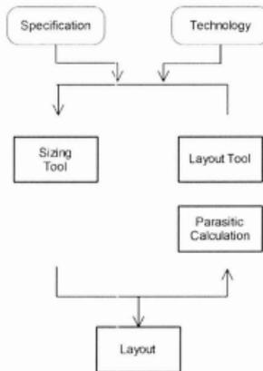
Figure 8: Layout-oriented synthesis proposed in [12].
