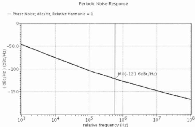
**Figure 63:** Phase noise at 600KHz for approx. total capacitance of 251.29fF for LC Oscillator in *TSMC 90nm* technology that yields oscillation 5GHz.
