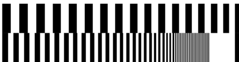
Figure 2: The Camera Resolution and Imagery Board (CRIB) adapted from the 1951 USAF resolution test chart [Department of Defense, 1959] consisting of 72 black bars ranging in width from 0.1-8.0 cm to test the image quality of the underwater camera systems.
