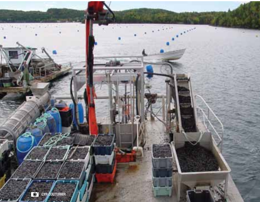
Figure 2: Blue mussel farm in Notre Dame Bay, Newfoundland. Mussels are suspended in the water column using longline technology; they filter-feed on natural ocean plankton; and vessels grade and harvest using hydraulics/automation.
