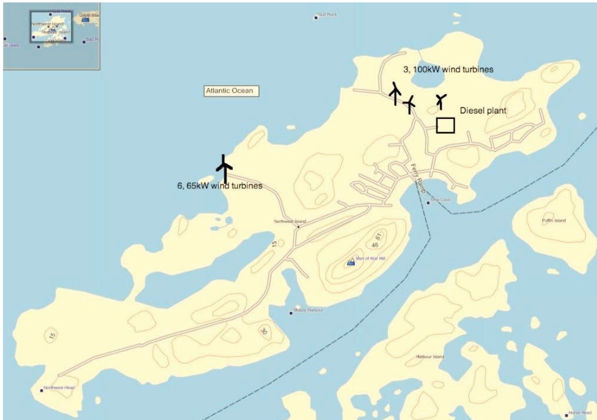
Figure 4: Location of wind turbines and diesel plant in Ramea
