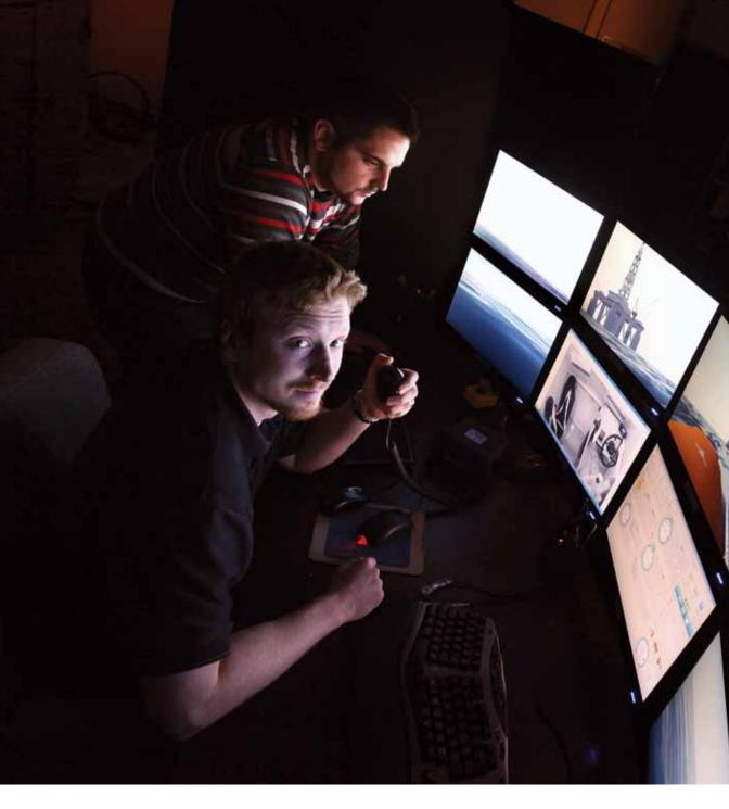
The freefall lifeboat simulator was built as a collaborative research project between the Faculty of Engineering and Applied Science at Memorial University of Newfoundland and Virtual Marine Technology Inc. (VMT) and is the only DNV accredited freefall simulator in the world. The simulator replicates the coxswain's position and two crew positions in
