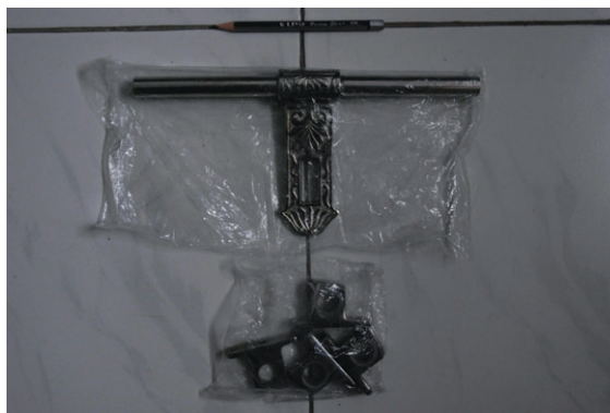
Plate 1 A lock for a gate manufactured from former e-waste and other metal scraps in Dhaka, Bangladesh
