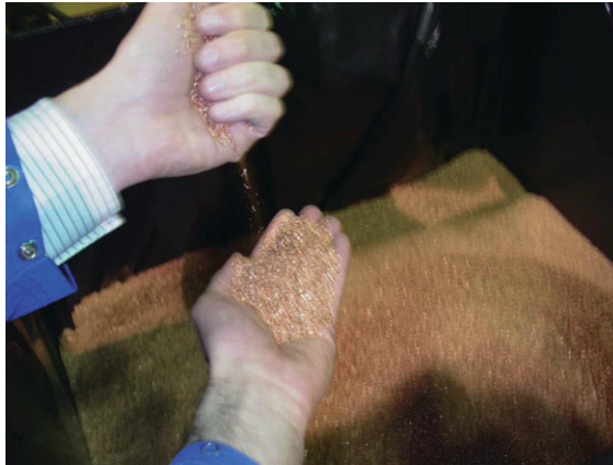
Plate 2 Former e-waste processed into commodity grade copper
