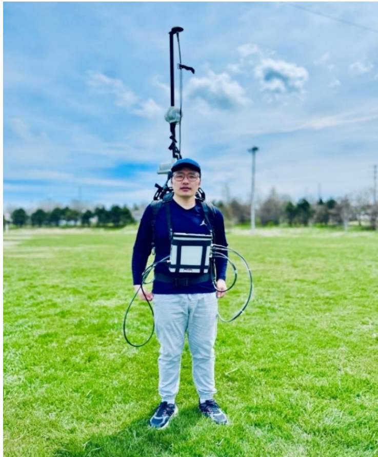
Figure 3.3: Overhauser magnetometer assembly deployed at the site.
