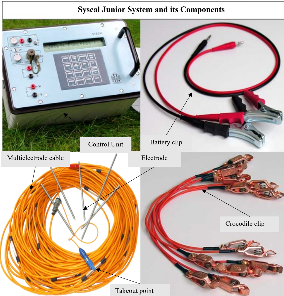
Figure B.4: Components of the Syscal Junior system from Iris instruments used in this work.
