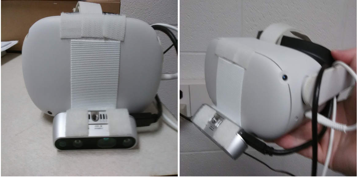
Figure 3.8: Experimental Setup, Left: the front view displays the camera mounted on the headset, with the camera's position relative to the headset being adjustable.; Right: Side view demonstrating the dynamic adjustment of the camera angle, oriented to facilitate a comfortable position for the user to hold the phone in front of the camera.
