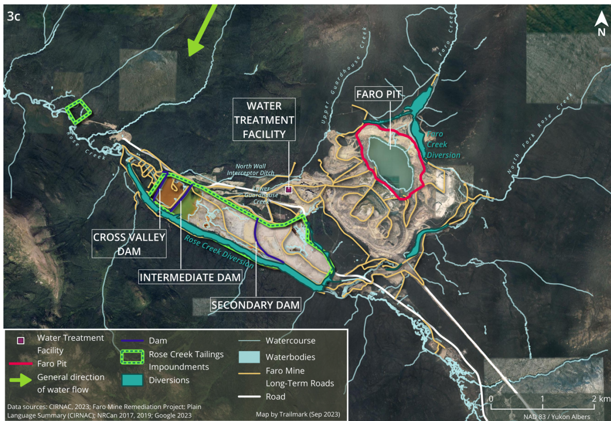
Figure 4.3 Map of the water flows through and diversions around the Faro Mine site. Trailmark, September 2023
