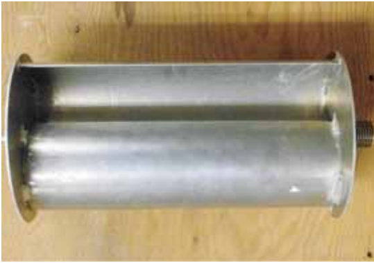
Figure 1: The experimental Savonius rotor.
