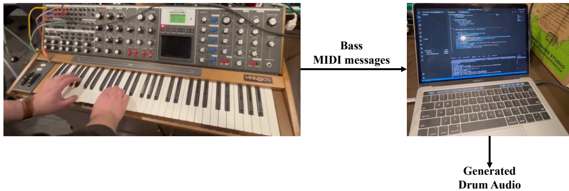
Figure 4.1: Setup of a human interacting with the drum companion. For the ease of generating MIDI messages, we used a MIDI keyboard instead of a bass guitar. The computer runs the DG model and plays the output, the generated drum track, to accompany the human player. To reduce generation latency, we did not use VA in real-time interaction.
