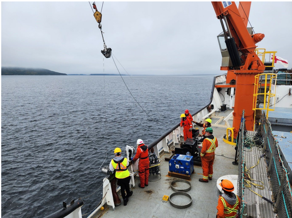
Figure 7: Van Veen sample deployment from the post side of the MV Polar Prince using the scientific winch and crane (photo from Alexandria Fudge).
