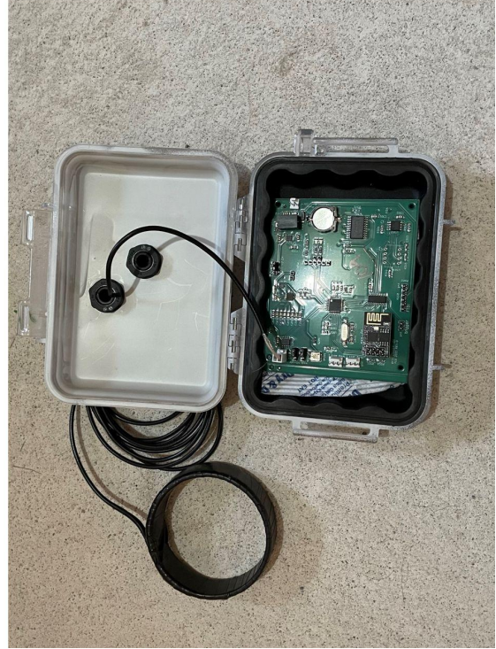
Figure S2. (A) Leach's Storm-Petrel equipped with a PIT tag contained within a custom 3D-printed leg band. (B) PIT tag system including the tag reader (black circle) which is inserted into the mouth of the burrow.
