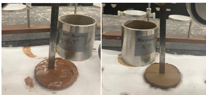
Fig. 13: Filtration test mud cake for imaging fluid produced using 3000 rpm (+ oven heated for API barite) mixed at low temperature.
