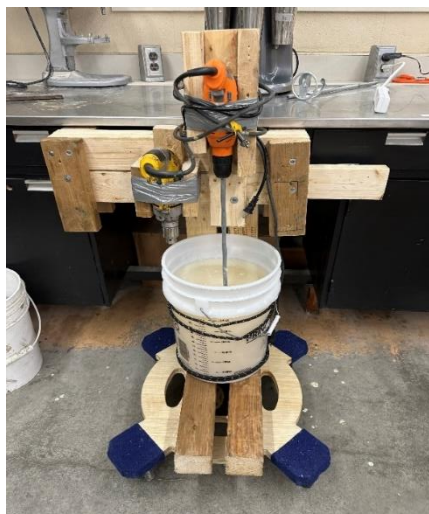
Fig. 1: Hand drill mixing blade and experimental setup.
