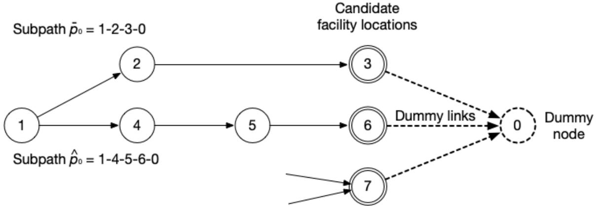
Figure 4.1: Convert from LNDP to PNDP (adapted from Liu and Kwon (2020))
