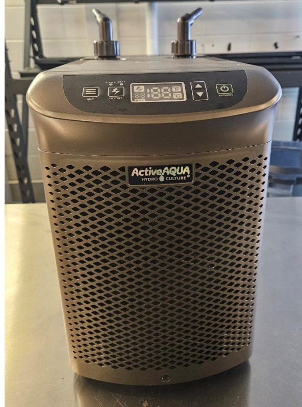
Figure 3.3. ActiveAqua AACH10HP water chiller used to chill a tank of water containing TTLCs to 4°C and 12°C.
