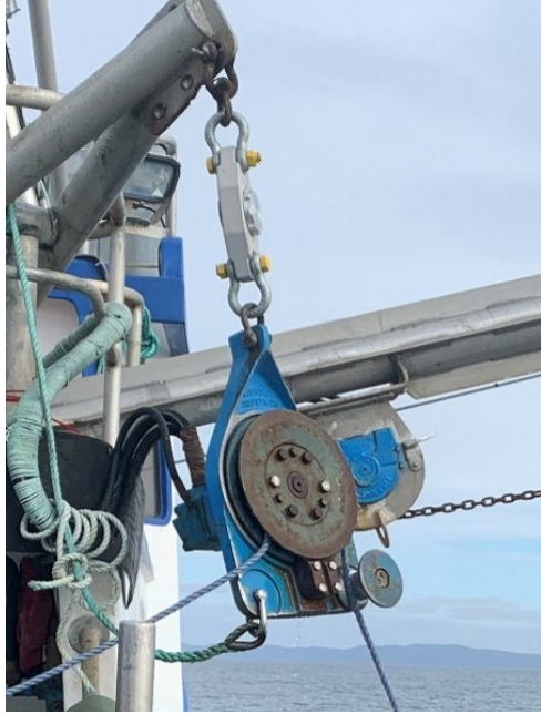
Figure 2.4. Picture of the Euroload load-cell (ELT24) installed above the hauler aboard the FV Island Voyager fishing vessel during the experiment.
