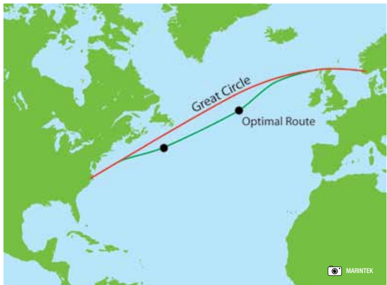
Figure 2: Great circle sailing versus weather routing on a typical trans-Atlantic voyage.
