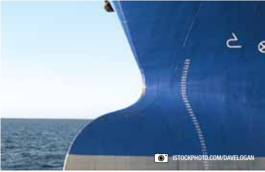
Figure 6: A bulbous bow is a tubular shaped piece protruding from the stem of a ship that changes the hydrodynamics of a moving vessel. Developed by David Watson Taylor in 1910, the design has been developed and streamlined to provide optimum performance for a ship.
