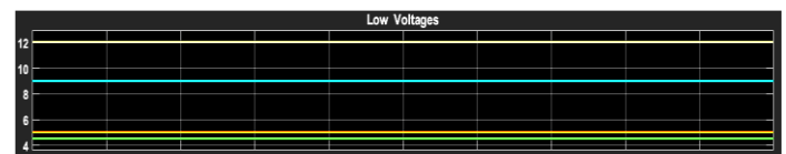
Fig 7: 12 V, 9 V, 5 V and 4.8 V output voltages.
